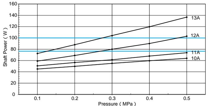
Select the best motor using the lines in the "Required Power" table as the applicable standards.
